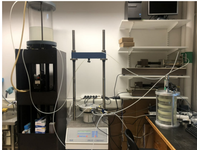
Figure 4.2: Triaxial test setup in LTH Geotechnical Laboratory
