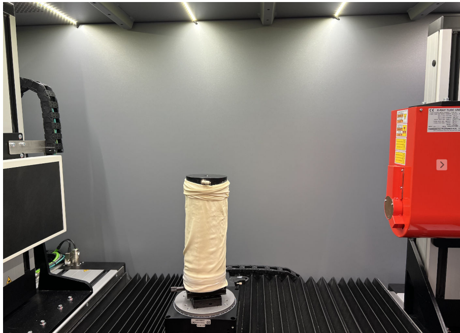
Figure 6.1: Image acquisition via XRT in 4D Imaging Lab
